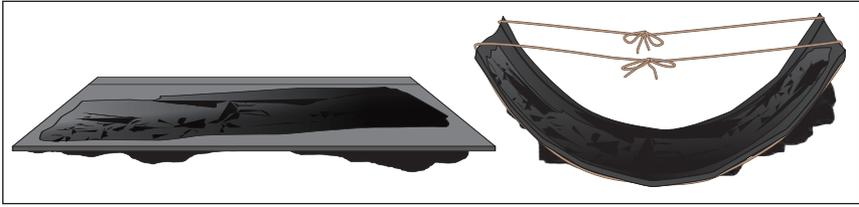
Once you are happy with the shape of the mold and it is held firmly in place, mix the plaster to a paste-like consistency. Apply the plaster by pushing the plaster into the vertical curved areas with a craft stick or brush. If using string to hold the mold in a U-shape, you can also roll the mold to the left and right and let the plaster ooze into the vertical corners. Let cure overnight before removing the rock from the mold. Peel the Rock Mold off of the rock gently.
