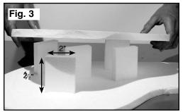
BASE aside. Draw a 3" square around "X" and cut out section on LOWER BASE. Glue all SUPPORTS, 2" side down, to the LOWER BASE (Fig. 3), keeping the supports one inch in from the traced edge of the UPPER BASE (Fig. 1). Next, glue the UPPER BASE on top of the supports, lining up with the traced lines and let the glue dry (Fig. 3).
