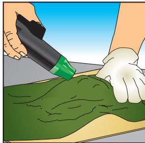
Wear the Forming Glove provided and form the mat using the Heat Tool.
