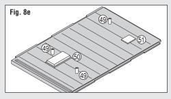
Roof (Fig. 8e) Vents x3 49, Large Hatch 50, Small Hatch 51
