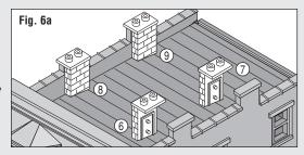
**IMPORTANT** Assemble and install Details using Cyanoacrylate Adhesive (CA glue / super glue). If Details were left on sprue while painting, remove using a hobby knife (or flush cutting shears). Sand parting lines and touch-up with paint. Details have unique placement posts for predetermined locations. Test fit Details before gluing.
