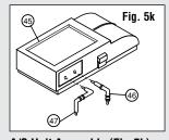
A/C Unit Assembly (Fig.5k): Assemble and glue A/C Unit, (4) A/C Elbow Pipe (40), Double Elbow Pipe (47). Glue A/C Unit Assembly to Building.
