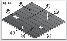
Roof (Fig. 6e): Hatch ③, Small Vent 2x ③, Tall Vent ③, Square Vent ④, Small Exhaust Pipe ④, Exhaust Pipe ④
